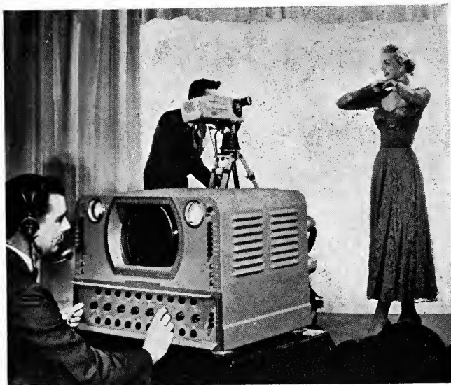
Fig. 32. Industrial color television equipment; camera and control console.
